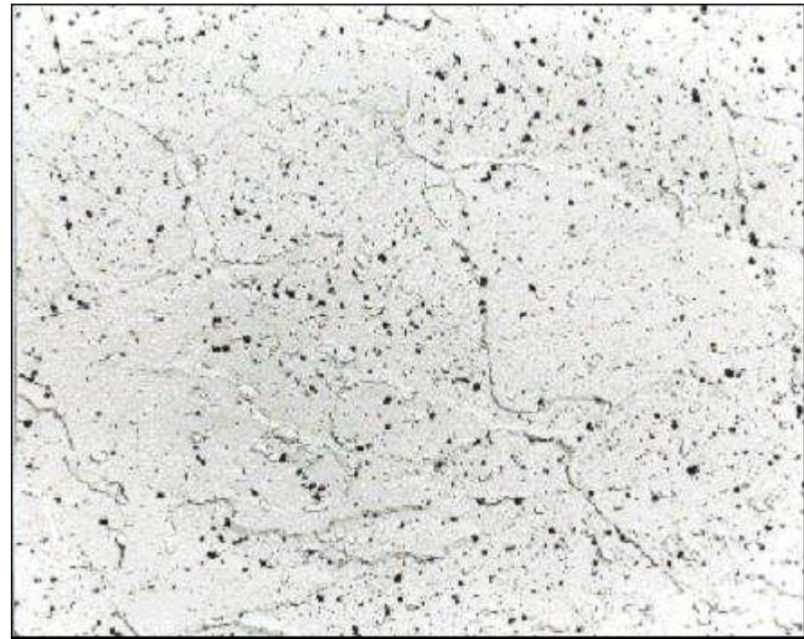
Węgliki \text{M}_7\text{C}_3 , \text{M}_{23}\text{C}_6 , \text{M}_6\text{C} i \text{M}_2\text{C} w stali 2,25Cr-Mo-0,25V (M=Fe, Cr, Mo, V). TEM
