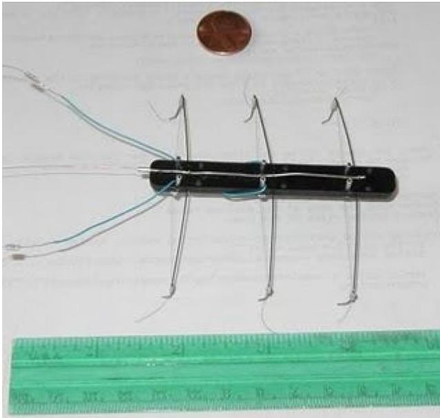
*In aircrafts they are developed a gadget called Variable Geometry Chevron using shape memory alloy that reduces aircraft's engine noise.*
